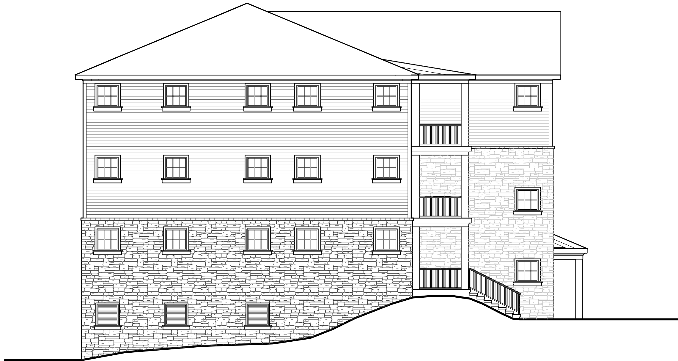
① Left Side Elevation Lot 3 Scale: \frac{1}{8}'' = 1'-0'' Left Side Elevation for Lots 2 and 4 is similar.
